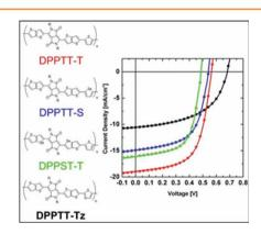
Four diketopyrrolopyrrole containing polymers are synthesized and evaluated for use in organic solar cells. Heteroatomic substitution allows precise control over the polymer energy levels with minimal disruption to the solid state properties. Variations in the short circuit current are linked to the energetic offset between polymer and fullerene.
