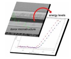
The influence of intraphase microstructure on the performance of organic photovoltaics (OPVs) is studied utilizing a bilayer (planar heterojunction) device architecture. Devices in which the donor layer exhibits subtle differences in microstructure are compared, and these differences are shown to affect critical parameters (energy levels, charge transport properties) having a significant impact on performance.
