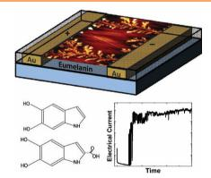
Thin films of the biomolecule eumelanin interfaced with Au electrodes lead to the growth of Au-eumelanin dendrites and show a resistive change under prolonged electrical bias. This phenomenon, partially attributable to the metal chelation properties of eumelanin, has to be considered in the design of eumelanin-based bioelectronic devices.
