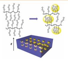
A new series of polymers containing  $\pi$ -conjugated oligomer as side chains show great promise as candidates for high performance nanodielectric materials. The oligomer-based highly polarizable side chains can self-organize to form nanoscale, conjugated, electrically conductive domains, which uniquely meet the requirement for nanodipole architecture, resulting in high permittivity and low dielectric loss across a wide range of frequency (100 Hz-4 MHz).
